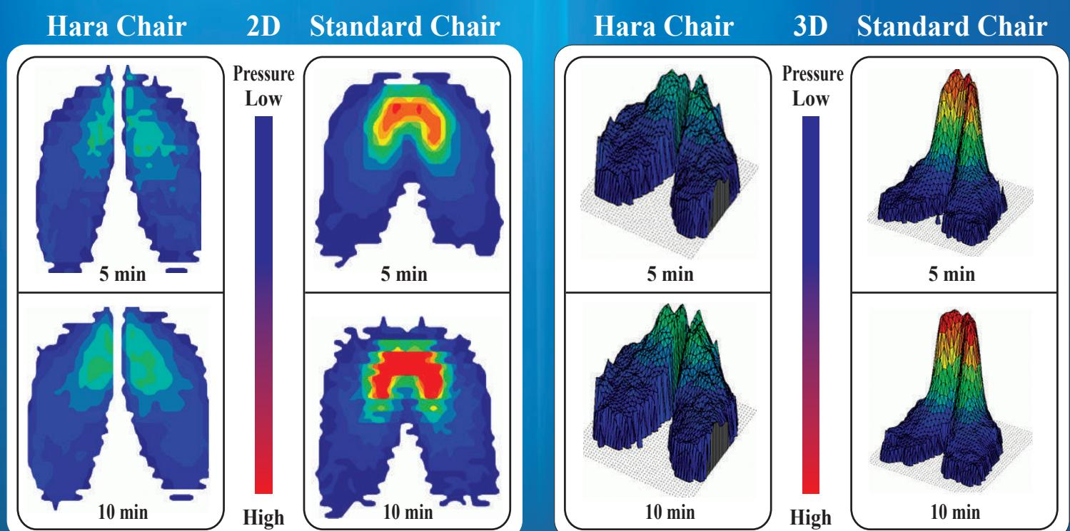
Pressure measured in tests at the Orthopaedics & Rehabilitation Institute for Technical Research.
